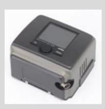
The H1D can be used untethered or tethered. 'Untethered' means that the camera is connected only to its Image Bank which acts as an image storage facility and power supplier to the sensor unit ( the camera body, viewfinder and lenses take their power requirements from the batteries in the grip). 'Tethered' means that the combined camera and Image Bank are connected to a computer.
