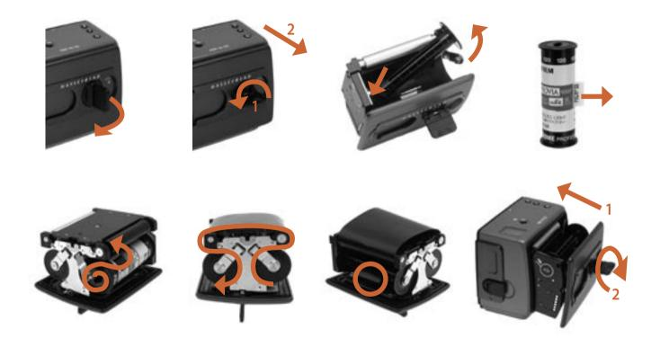
key clockwise 90° to lock the film holder in place and fold the key back into its stored position. You might find that increased pressure on the left hand side of the film holder will more easily ensure a positive and correct positioning in the magazine.
