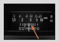
In the illustration given here, the focusing distance is set at nearly 3 metres. At an aperture of f/22, the depth-of-field would therefore extend from just over 2 m to approx. 4.5 m.
