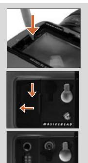
Do not attempt to clean the screen by immersing it in water, or use any kind of cleaning fluid. If the screen becomes damp, do not use hot air to dry it. Use a soft cloth on the upper surface only. Seek advice from an Authorized Hasselblad Service Center if the screen becomes particularly soiled. Remember that particles or greasy marks on the screen might impair the viewfinder image but have no effect whatsoever on the recorded image.
