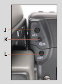
On the rear of the grip, as well as the rear control wheel, there are also a further three control buttons:
