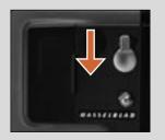
To raise the flash unit into its operative position, slide the flash-unit catch backwards in the direction of the flash symbol. To return the flash unit into its closed position, push down on the top of the unit until it clicks back into place. The flash unit is automatically activated when it is in the operative position and de-activated when returned to its stored position.
