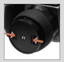
by unscrewing it in a counter-clockwise direction. Align the index on the lens with the index on the camera body and rotate the lens clockwise (bayonet fitting) until it clicks into place.
