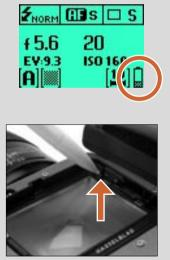
the locked position. Holding the battery holder flat against the grip and aligning the two upper lugs with the slot in the grip, slide it back into position as far as it will go. Swing back the battery holder retaining lever as far as it will go into the locked position.
