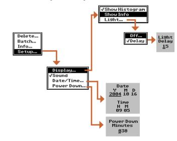
Use the **Display -> Show Histogram** and **Show Info** settings to display the histogram and info bar respectively for the current image on top of the preview image - see 'Displaying Images'. Use the **Display -> Light...** setting to turn the display background light on or off. When using the **Delay...** function the light is set to automatically turn off after a certain time of inactivity.
