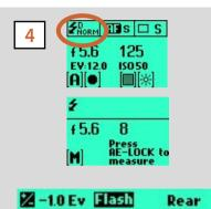
Example of viewfinder LCD display showing Flash set to Rear sync as well as - 1EV exposure compensation.
