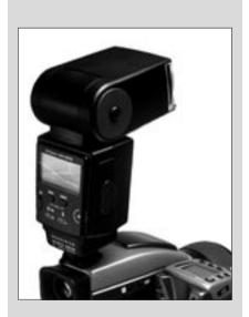
The H1D can be used together with most flash units. Connection is either by the PC socket or by the hot shoe if the unit is compatible (see note below).
